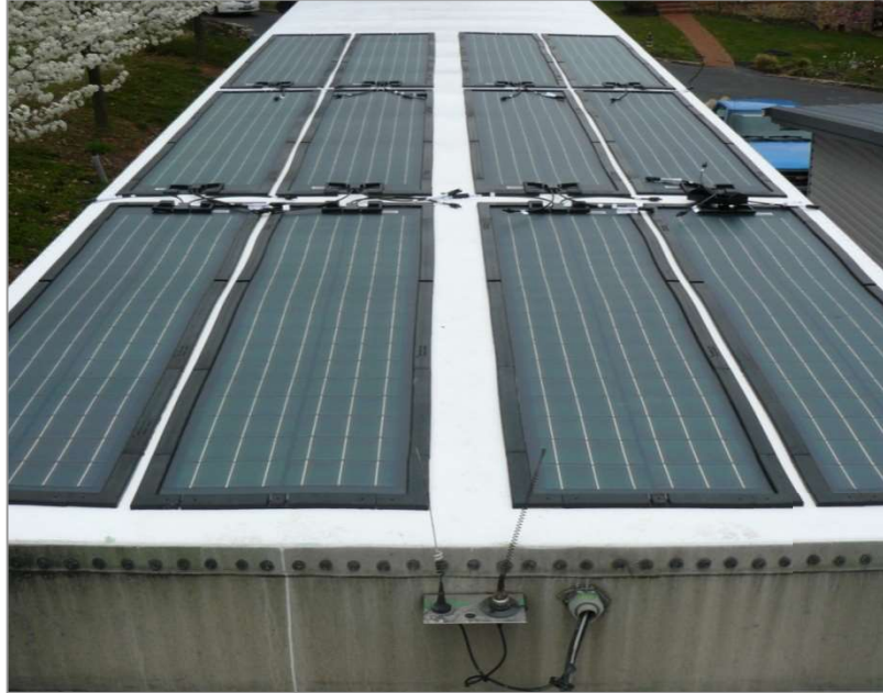
Application of CIGS Flex modules on refrigeration trailer
