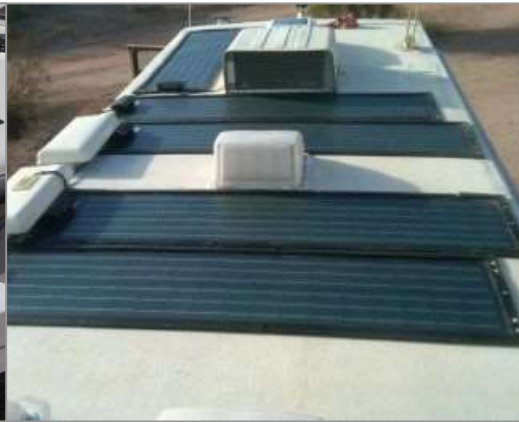
Application of CIGS Flex modules on RV roof
